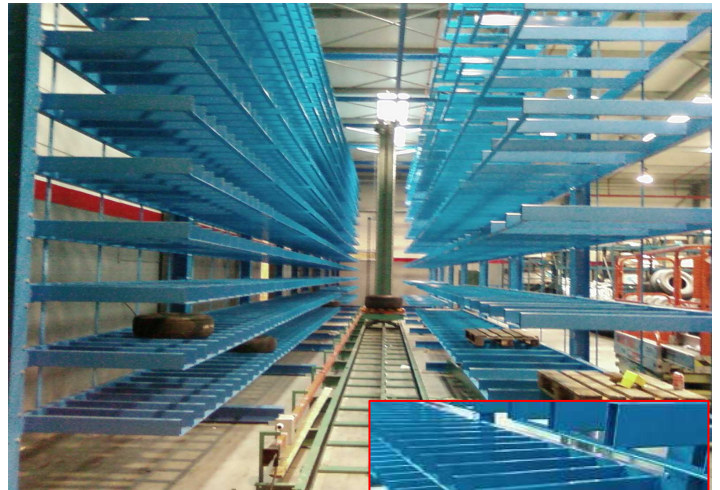
Storage of airplane tires with automatic loading.
